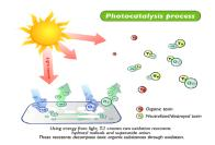
New photo catalyst LiNbO3for Corrosion Reducing and Environment Friendly Sustainable Concrete Construction.
