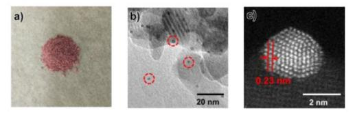
of gold nanoparticles through Scanning Electron Microscope.
