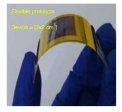
Fig.1: Electrodeposition of PEDOT film on flexible PET; Image- flexible electrochromic device
