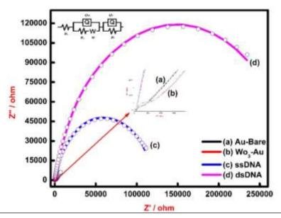
Figure 1- Electrochemical impedance behaviour of Modified gold electrode measured in PBS buffer (pH 7.4) in presence of 1mM  $K_3/K_4$  Fe[(CN)<sub>6</sub>]<sup>3-/4-</sup> in the frequency range of 100KHz to 1KHz and applied potential 0.16v.
