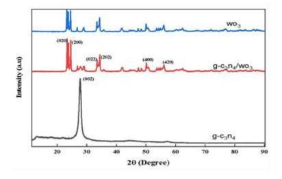
Figure 1: Comparison between the measured XRD pattern of g-C3N4, WO3, and g-C3N4/WO3 composite synthesized via physical grinding for 2 h and heated at 500°C.
