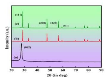
Figure 1: XRD pattern of (a) g-C3N4, (b) CeO2, and (c) g-C3N4/CeO2 composite prepared via physical grinding References:
