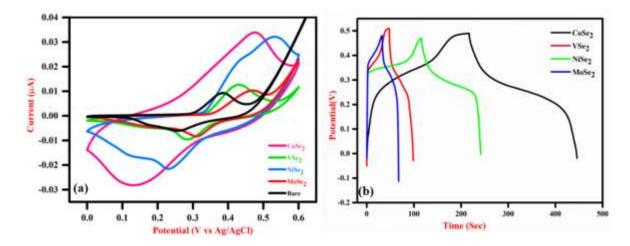
Figure: (a) Comparison of CV responses of bare NF, and TMS (M = V, Mo, Co, and Ni) at a scan rate of 50 mV/s and (b) Comparison of GCD curves of TMS (M = V, Mo, Co, and Ni) at 1.25 A/g.
