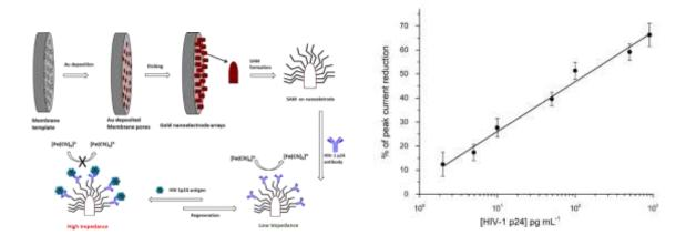
Fig.1 Schematic illustration of the different steps for the immunosensor construction
