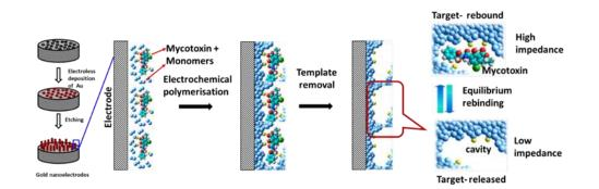
Scheme 1. Schematic representation of MIP sensor for Aflatoxin B1 fabrication and sensing mechanism.
